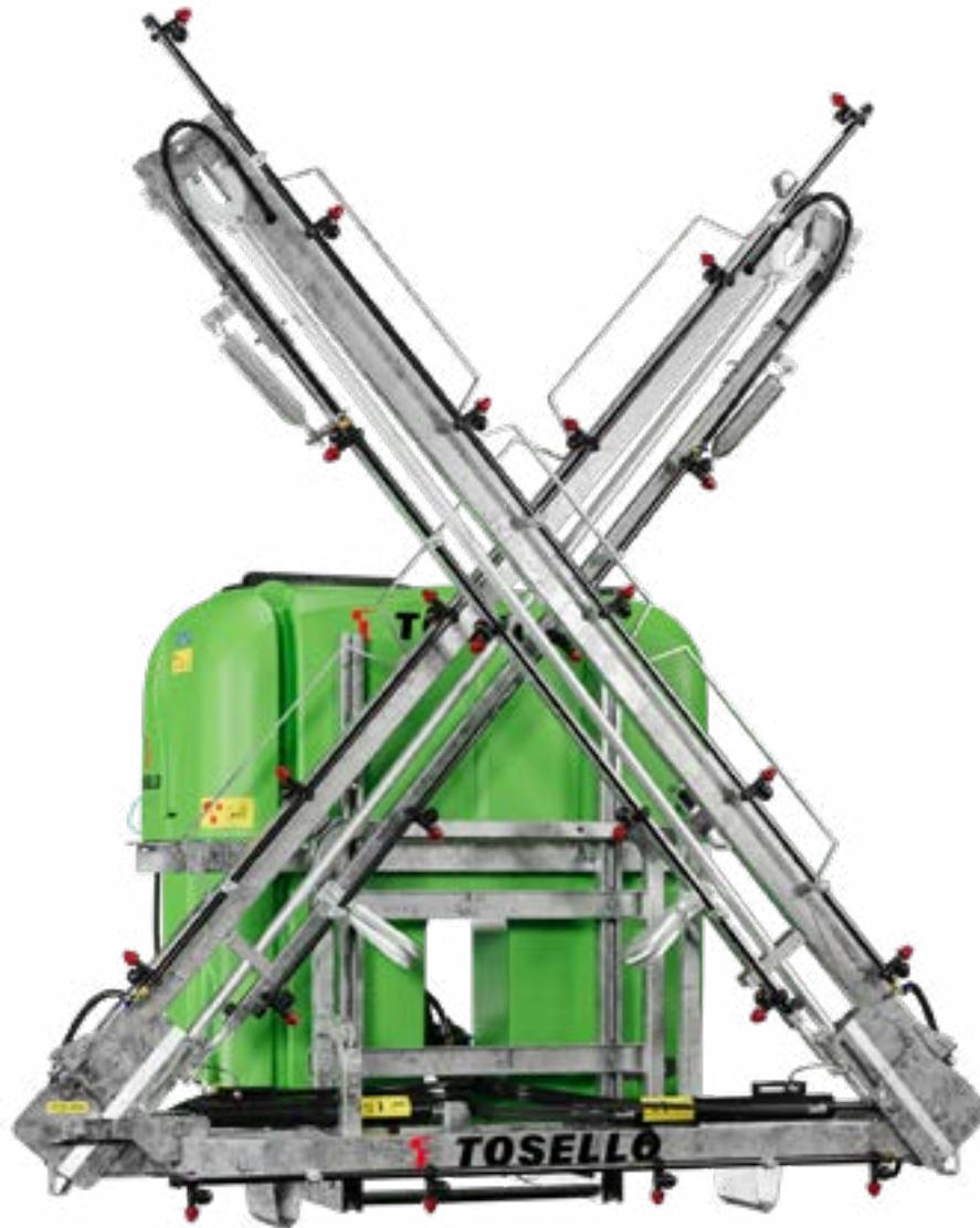
**Professional linkage sprayer for medium-large farms. It is just the right compromise between affordability and a quality product. This type of unit has a tank capacity ranging from 400 to 600 litres, and features an L2 hydraulic weed spray boom measuring between 6 and 12 metres in width.**
