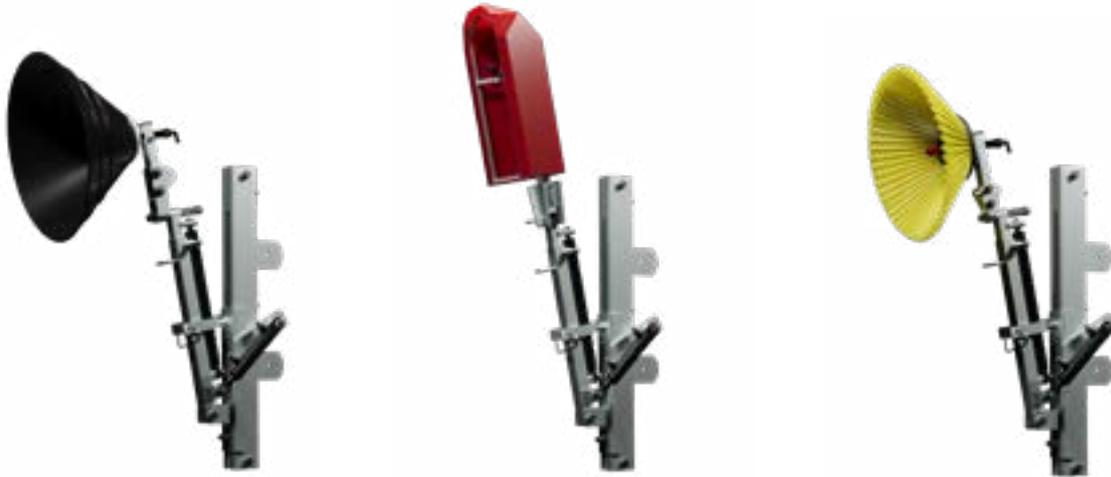
**Professional weed control unit. It can be configured to your requirements: height above ground as well as angle, spray head opening and extension can all be controlled directly from the tractor's cab.**
