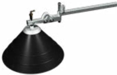
Zinc-plated metal structure, spring-loaded break-back, Ø 500 rubber cone, AISI 304 stainless steel nozzle holder, fixed plastic nozzle, Kematal 03/110 nozzle tip.
